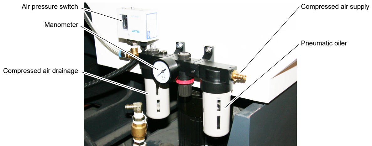
Img.3-7: Compressed air maintenance unit
