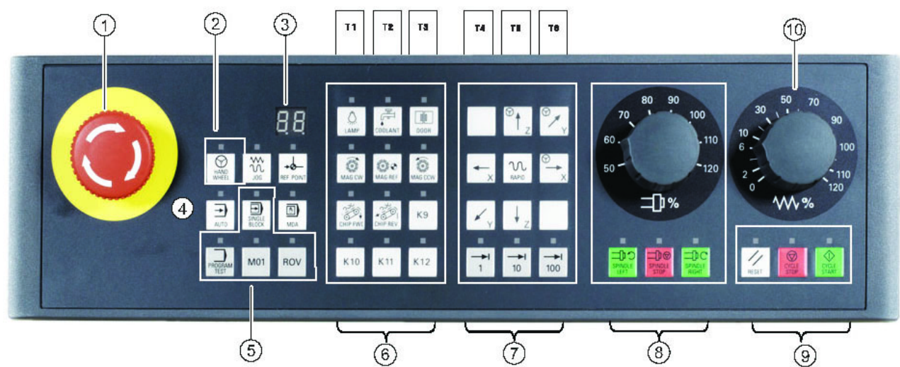
Img.5-3: Machine Control Panel
