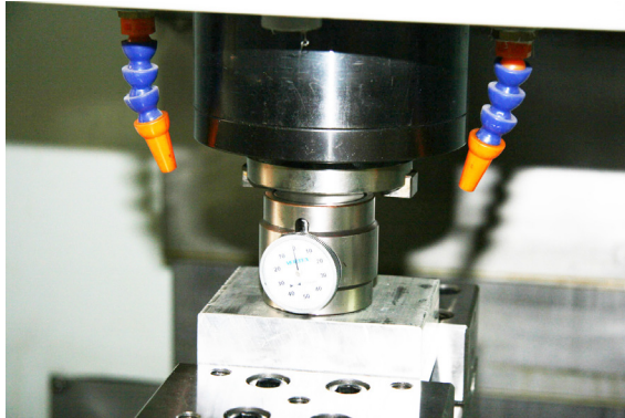
Img.6-6: Workpiece datum Z axis with pressure sensor
