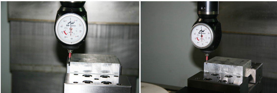
Img.6-5: Determine workpiece datum X axis resp. Y axis
